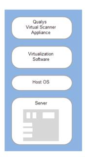
Qualys Virtual Scanner Appliance is packaged and qualified for deployment on a variety of virtualization and cloud platforms.
