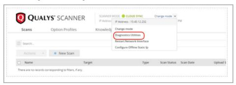
On the Diagnostics Utilities screen provide the IP address or DNS name of the scan target and then click Ping or Trace Route.
