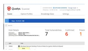
This is where you launch scans and manage your account data (option profiles, scan results). The web user interface can be accessed using any standard web browser (e.g. Internet Explorer, Chrome, Firefox) running on the host OS. The virtual NIC for the web interface should be deployed on a host-only network between the host (e.g. Windows) and the appliance virtual machine.
