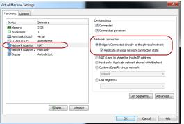
Configure virtual machine settings. For "Network Adapter", select the Bridged network connection and "Replicate physical network connection state". Save your settings.
