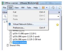
Bridged mode is required for offline scanning. To configure bridging in VMware, go to Edit > Virtual Network Editor.
