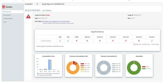
The Build Summary provides a dashboard view of your security posture. Go to Vulnerabilities for a list of detected QIDs, Installed Software to see software detected on the container image, and Layers to view a list of layers the image is made of.
