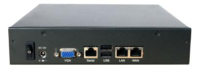
The Scanner's back panel includes: a power switch, a power socket, VGA socket, two USB ports, Ethernet LAN and WAN ports. (Note - The "Serial" Ethernet port shown is not in use; there is no Serial support on this scanner. The only way to have scanner console access is to connect a monitor to the VGA port and a keyboard to one of the USB ports.)
